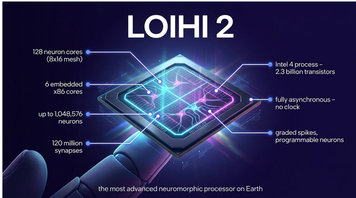
Figure 15. Intel Loihi 2: 128 neuron cores, ~1M programmable neurons, graded spikes, on-chip learning, on Intel 4.
