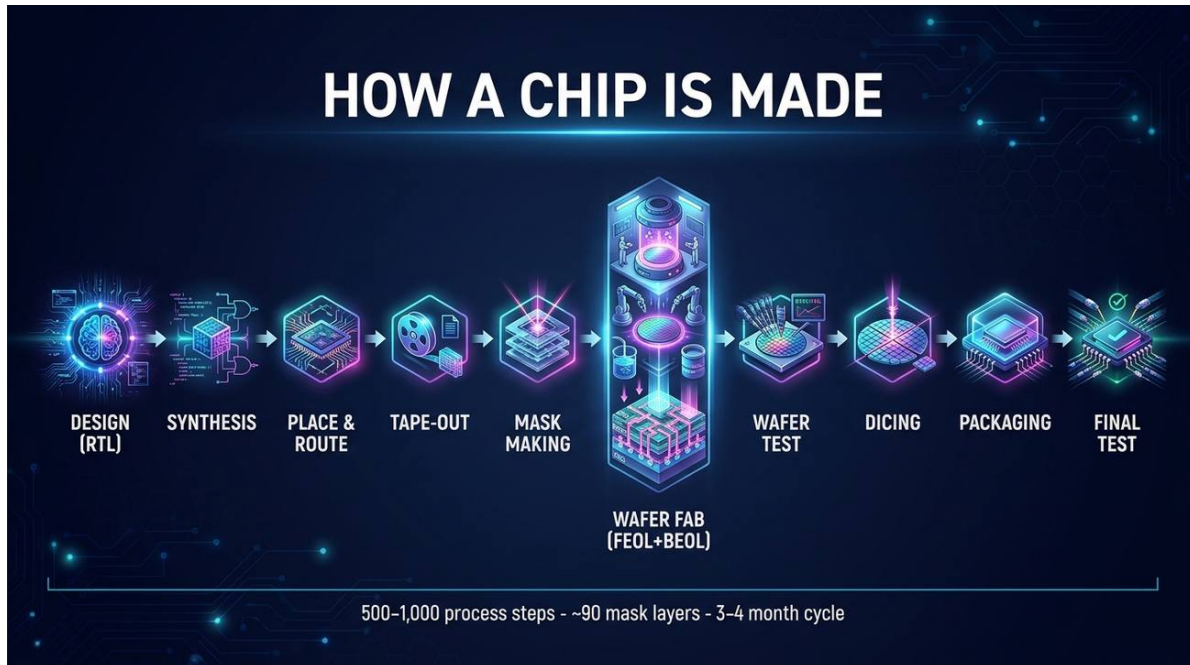
Figure 23. Making the chip: ~500-1,000 process steps and ~90 mask layers over a 3-4 month cycle.
